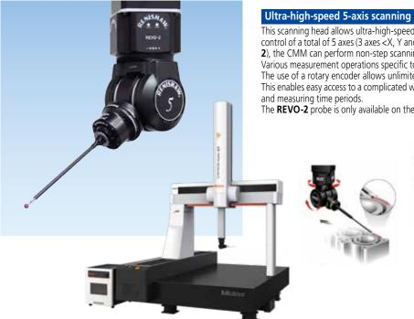
This scanning head allows ultra-high-speed scanning at up to 500 mm/s. With simultaneous control of a total of 5 axes (3 axes <X, Y and Z> on a CMM and 2 axes <A and B> on REVO-2), the CMM can perform non-step scanning of complex forms on a workpiece. Various measurement operations specific to REVO-2 are also available.
